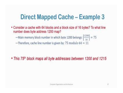
Now we take a third example: Consider a cache with 64 blocks and a block size of 16 bytes. To what line number does byte address 1200 map? So, the main memory block number in which byte 1200 belongs is given by 1200 divided by 16. Why? We have 16 bytes in each block and the block id is 1200. So, to which block number will this is will this byte 1200 belong it is given by 1200 divided by 16 which is 75.
